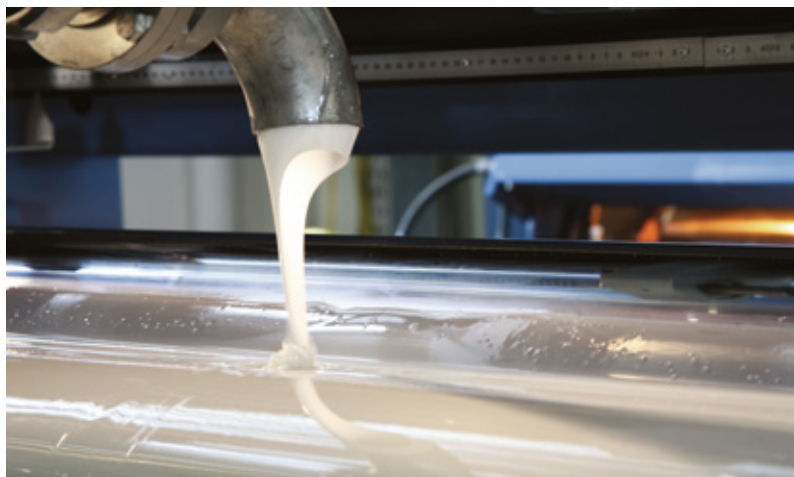
↑ Resin application for impregnation
